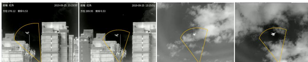
**Figure 13.** An example of narrowing the detection area by introducing prior information from radar. The yellow sector indicates the general location of the drone.
