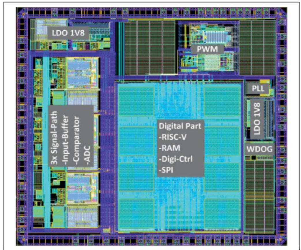
**Figure 9.** SoC layout with RISC-V architecture [110].
