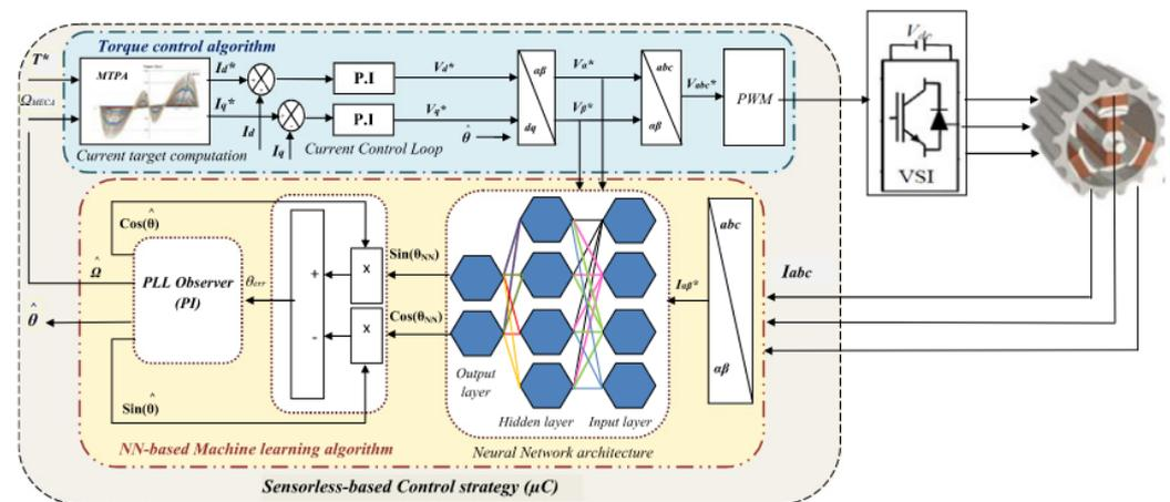
Figure 10. Structure of the IPMSM sensorless control based on AI [134].
