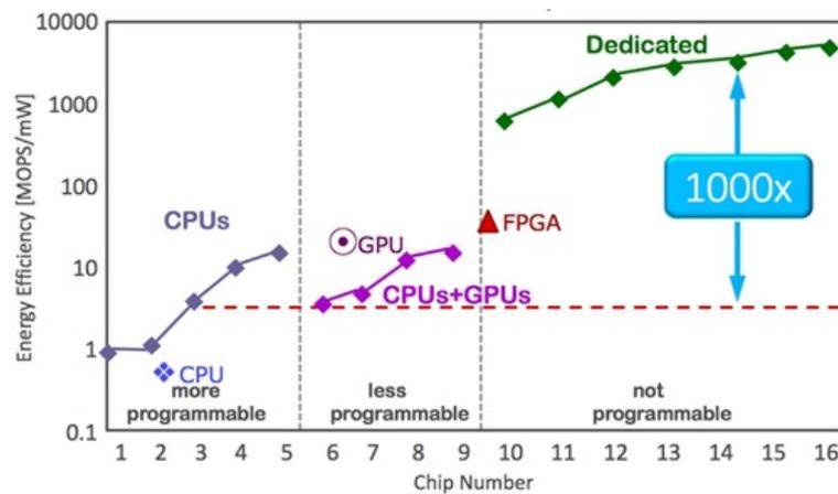
**Figure 2.** Programmability vs. Energy Efficiency [13].
