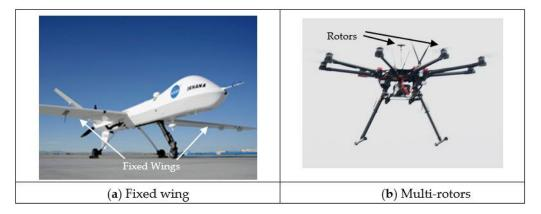
Figure 2. Commonly used UAV. (a) Fixed-wing UAV [29] and (b) multi-rotors UAV [30].
