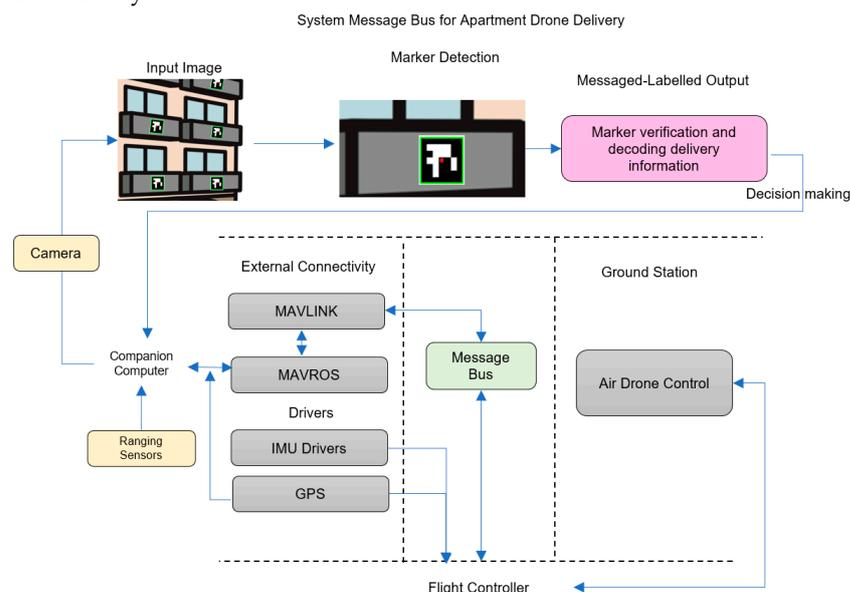
**Figure 6.** The block diagram to implement the marker detection for the drone system.
