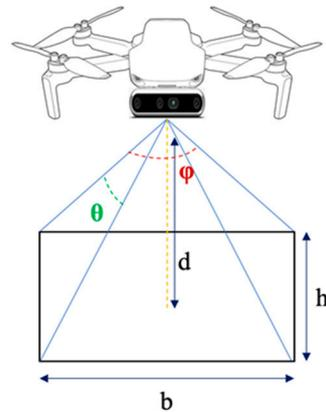
**Figure 11.** The drone camera's field of vision.
