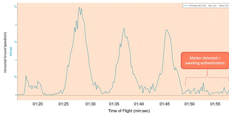
Figure 17. The horizontal ground speed data highlighting the section on drone marker detection and user authentication.
