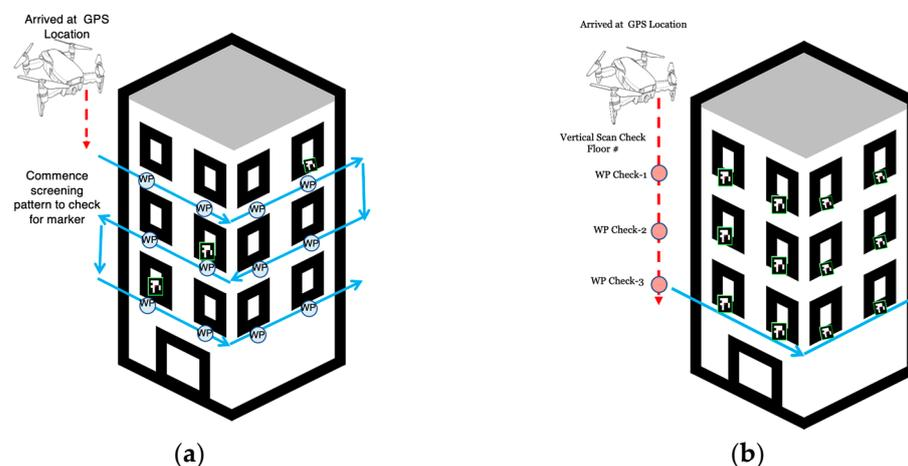
**Figure 2.** (a) The Grid Screening method; (b) The Square Screening method.
