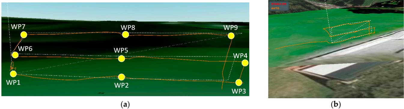
**Figure 12.** VGS Flight Test for Grid Screening (a) The GPS flight log illustrating the trajectory (orange line) of the flight and waypoints (in yellow) to scan apartments in a row. (b) The front view of the flight log in AUTO mode illustrates the executed trajectory.
