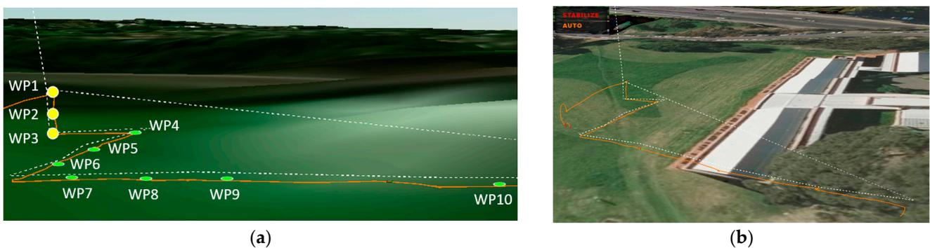
**Figure 13.** VGS Flight Test for Square Screening (a) The GPS flight log illustrating the trajectory of the flight (orange line) and waypoints (highlighted in yellow to scan for floor numbers and highlighted in green to scan apartments in a row). (b) The front view of the flight log in AUTO mode illustrates the executed trajectory.
