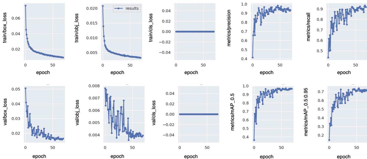
**Figure 8.** Mean Average precision and validation loss training result for four different 32-batch YOLOV5S models for approximately 4000 augmented images.
