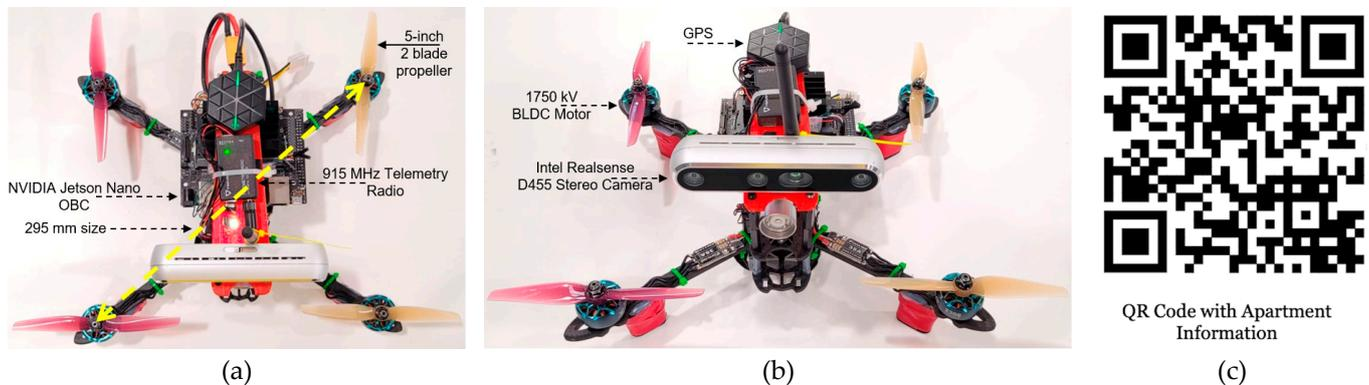
**Figure 5.** The photograph of the drone system assembled and ready for testing: (a) the top view of the assembled drone; (b) the front view highlighting the stereo camera used for marker detection; (c) the QR code with apartment information.
