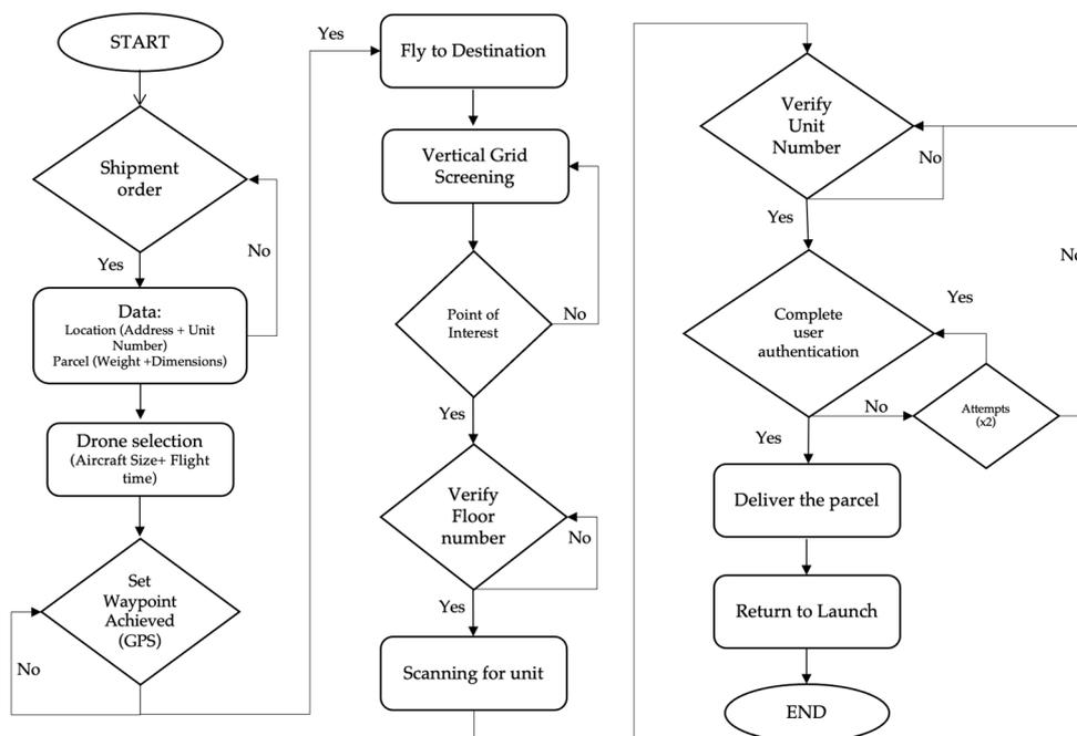
Figure 3. The flowchart of the proposed delivery for apartments with balconies.
