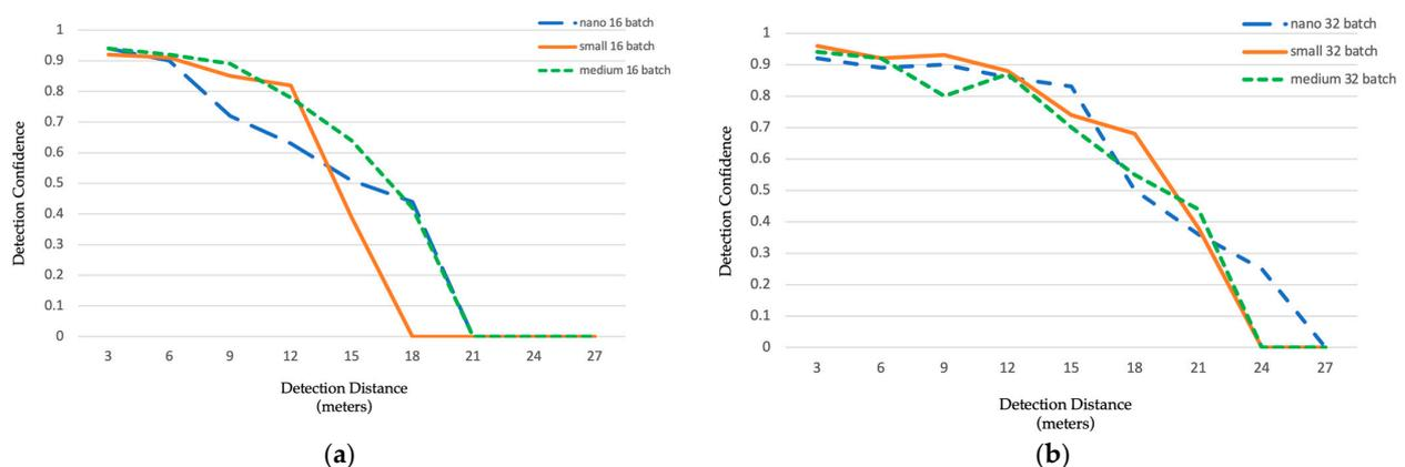
**Figure 9.** The following graphs illustrate the comparison results between three YOLOV5 (nano, small, and medium) models tested on the OBC of the drone system: (a) Confidence vs. Distance for 16 batch size model using  $480 \times 640$  pixels image resolution; (b) Confidence vs. Distance for 32 batch size model using  $480 \times 640$  pixels image resolution.
