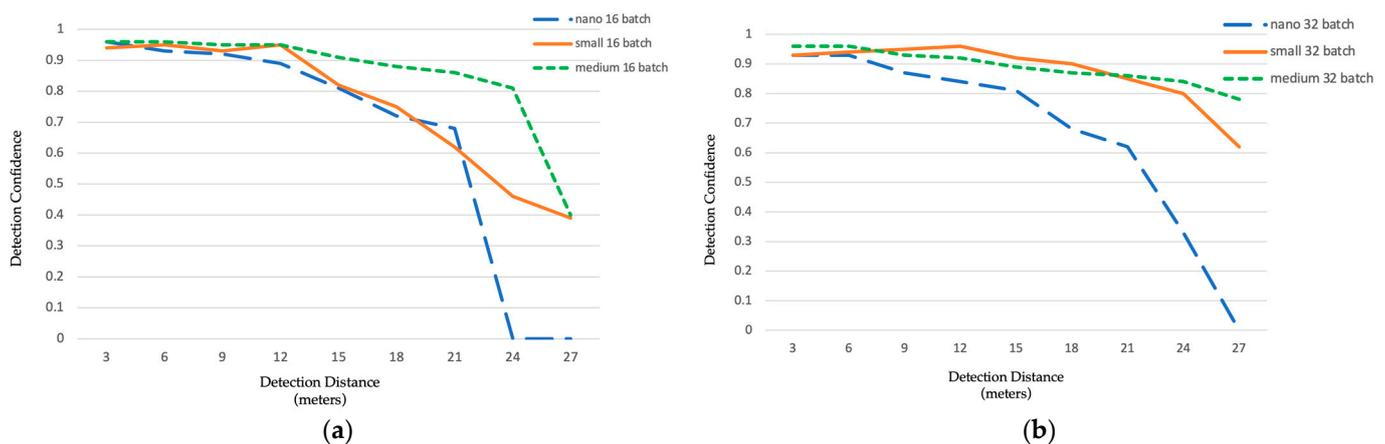
**Figure 10.** The following graphs illustrate the comparison results between three YOLOV5 (nano, small, and medium) models tested on the OBC of the drone system: (a) Confidence vs. Distance for 16 batch size models using  $960 \times 1280$  pixels image resolution. (b) Confidence vs. Distance for 32 batch size model using  $960 \times 1280$  pixels image resolution.
