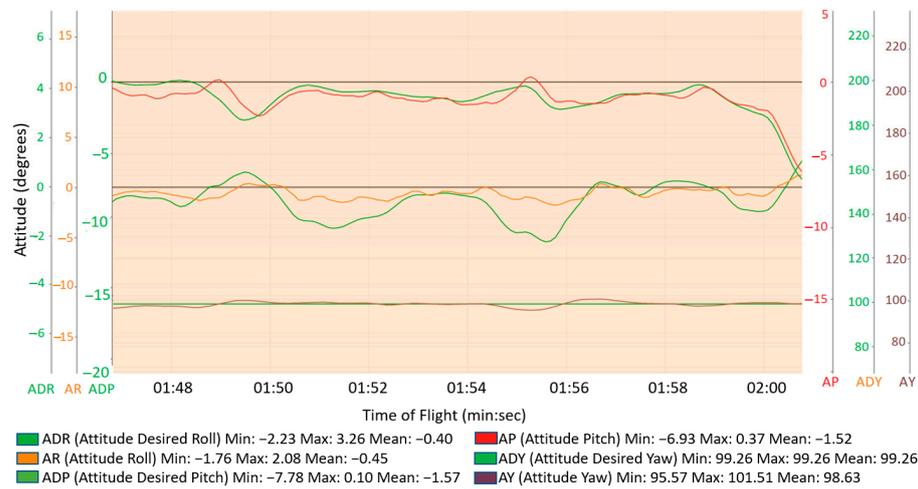
Figure 16. The flight log data of the drone mid-flight highlighting the actual vs. desired Roll, Pitch, and Yaw values for the Square Screening Pattern test.
