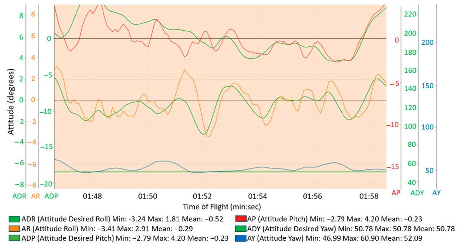
Figure 15. The flight log data of the drone mid-flight highlighting the actual vs. desired Roll, Pitch, and Yaw values for the Grid Screening Pattern test.
