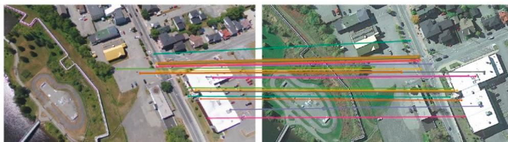
**Figure 2.** Example of feature point matching, UAV image (left) and satellite image (right).
