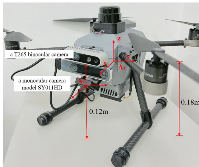
Figure 2. Mounting positions of the two cameras. The UAV's center, known as A1, is positioned on the frame's central axis, 0.18 m above the ground. The coordinates for A1 are set at (0 m, 0 m, 0 m). Meanwhile, the SY011HD camera's center, A2, is located at (0.08 m, 0 m, 0.06 m).
