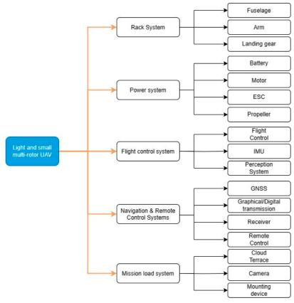
IMU:Intertidal Measurement Unit GNSS: Global Navigation Satellite Systems ESC:Electronic Speed Controller
