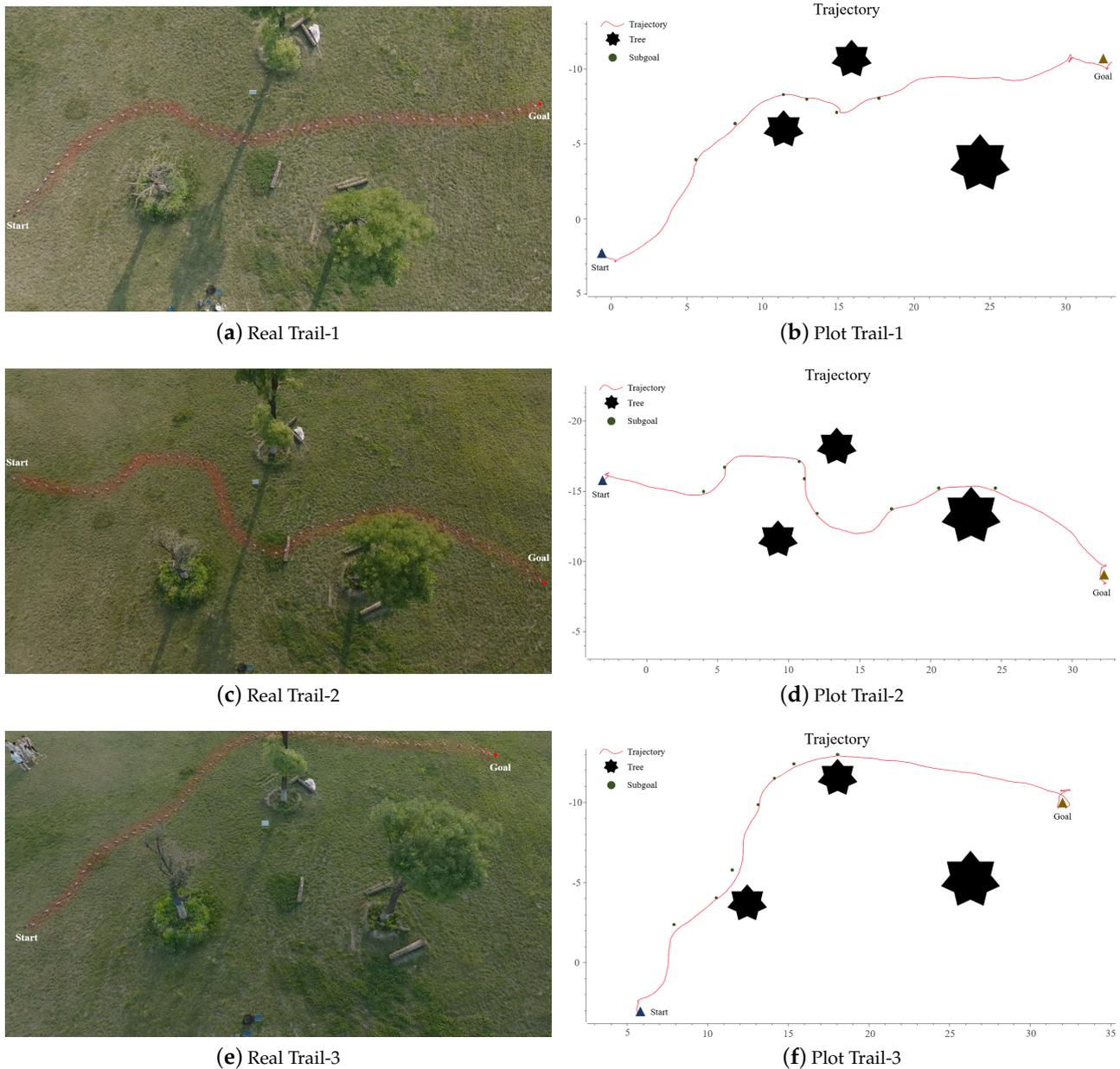
**Figure 11.** Real flight trajectories. (a,c,e) show the top view and (b,d,f) show the *Flight Log* plot trajectories of Trail-1, Trail-2, and Trail-3, respectively.
