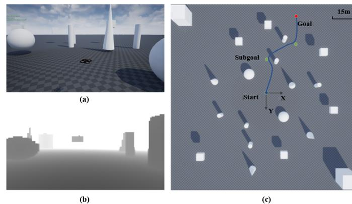
**Figure 3.** The simulation environment. (a) The simulator. (b) Depth image from the UAV view. (c) Top view of the environment.
