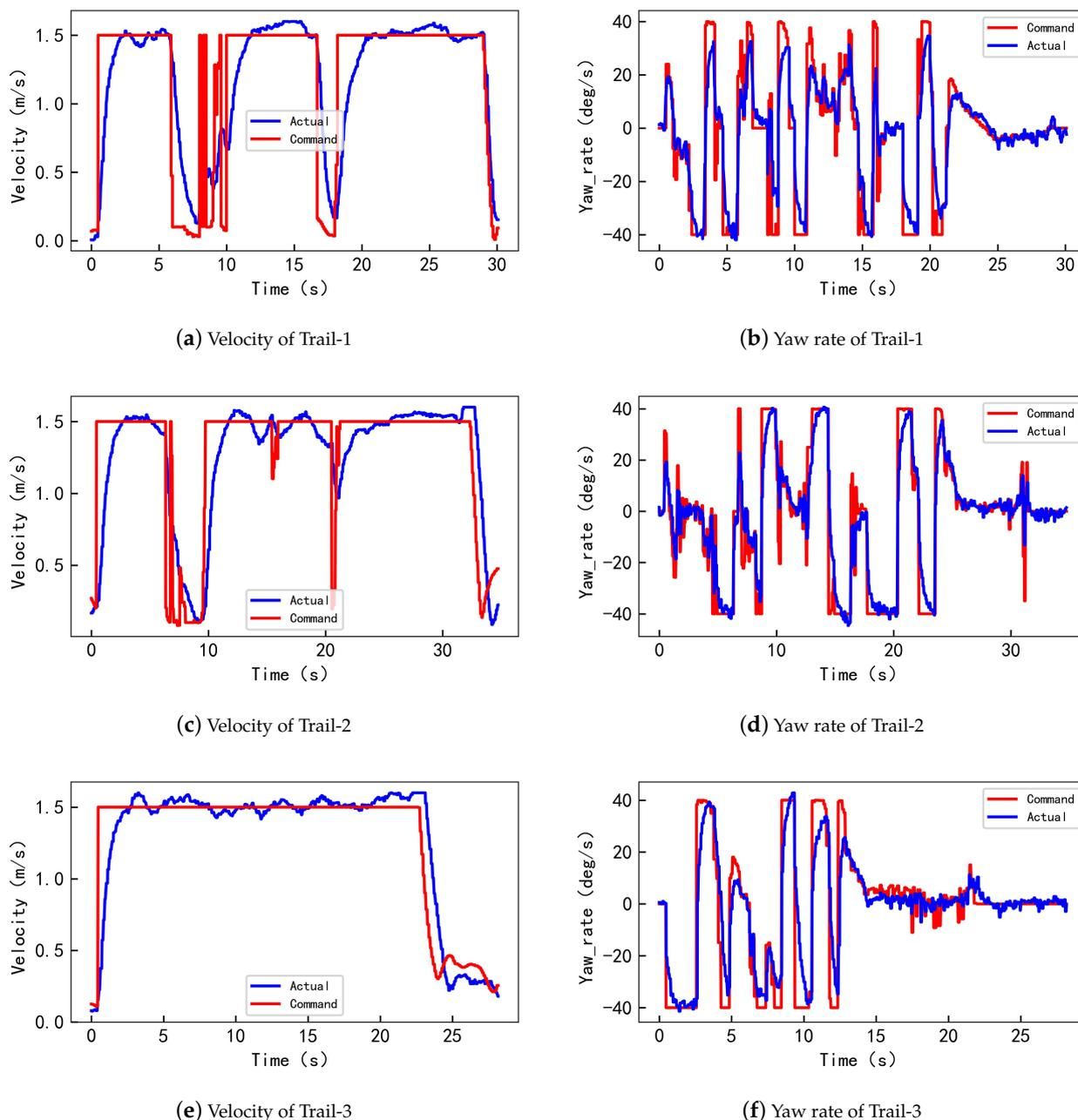
**Figure 12.** Real flight attitude. (a,c,e) show the change of velocity and (b,d,f) show the change of yaw rate of Trail-1, Trail-2, and Trail-3, respectively.
