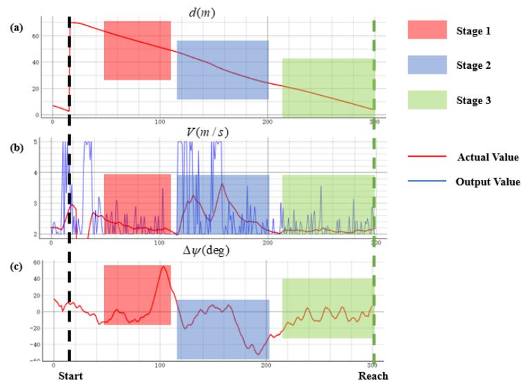
**Figure 9.** Dynamic states of the UAV with *Model<sub>700</sub>*: (a) shows the change of distance to the target; (b) shows the change in velocity; and (c) shows the change of yaw.
