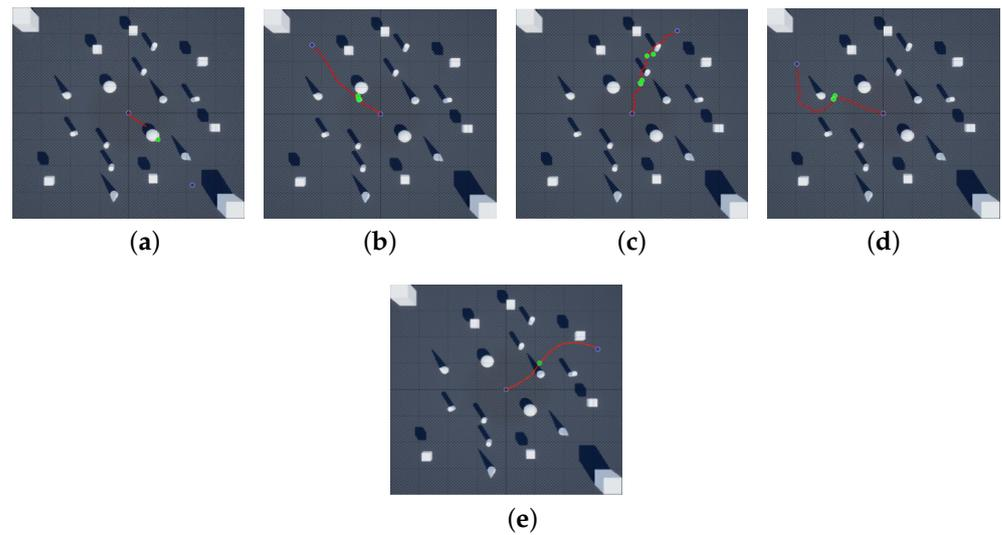
**Figure 8.** Performance of ETHP at different stages of training. The start point is located at the center of each graph, the red line shows the trajectory of the flight, and the goal point (blue dot) is randomly chosen in each episode. (a) 50 episodes. (b) 100 episodes. (c) 150 episodes. (d) 200 episodes. (e) 700 episodes.
