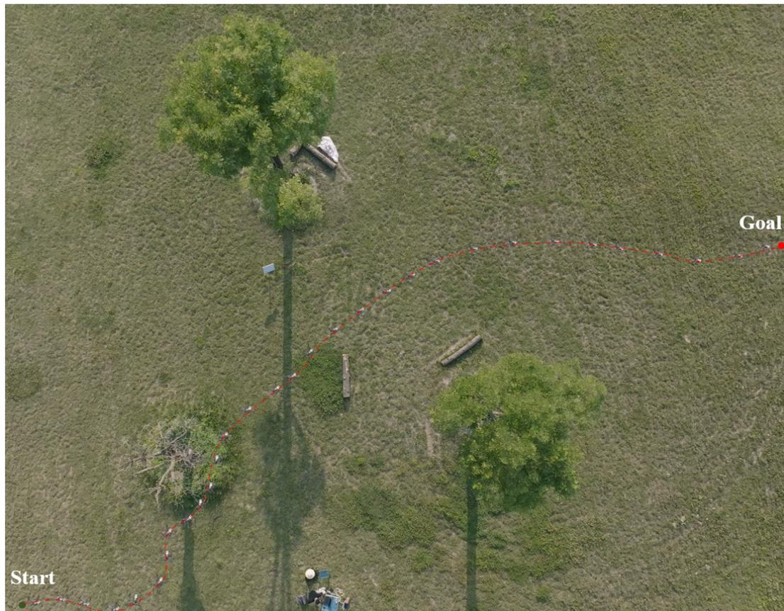
**Figure 5.** Real flight test environment. (the white dots in the picture are the positions of the UAV at different times captured by time-lapse photography, and the red line shows the entire flight trajectory).
