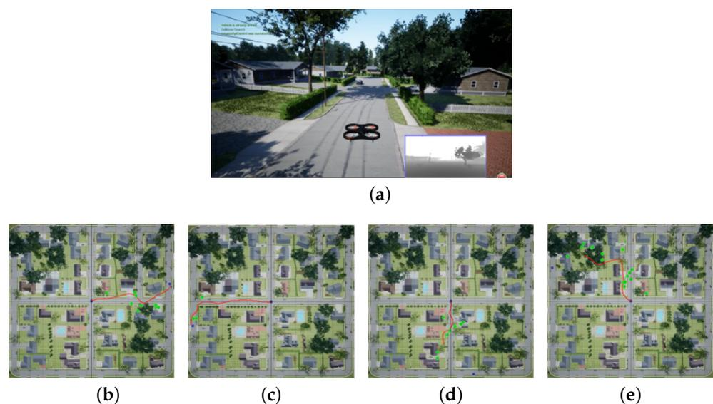
**Figure 4.** The performance of ETHP without tuning in the high-reality evaluation environment (includes different size of trees, houses, and poles). (a) Evaluation environment. (b) Trail 1 (success trajectory). (c) Trail 2 (success trajectory). (d) Trail 3 (crash trajectory). (e) Trail 4 (crash trajectory).
