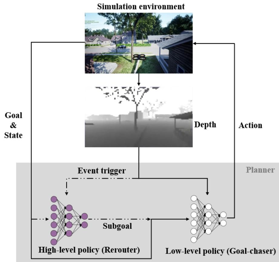
**Figure 1.** Event-triggered bi-level hierarchical planner (shown in the dashed frame). The planner directly maps from depth images to velocity and heading references. The high-level policy is triggered by the close obstacles and generates rerouting subgoals for collision avoidance. The low-level policy chases the (sub)goal.
