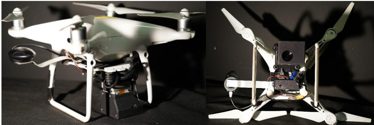
**Figure 2.** DJI Phantom 4 Pro with thermal sensor and custom mounting bracket. **(Left)** Front side view showing the custom mounting bracket attached to the underside. The external GPS custom aluminum bracket seen to the right-hand side of the airframe is clear of propellers and does not interfere with the onboard GNSS. **(Right)** Under view of the DJI Phantom 4 Pro.
