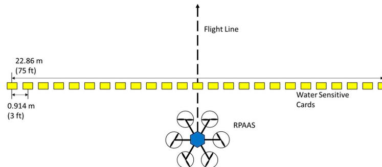
**Figure 1.** Layout of water sensitive cards and flight line during spray deposition measurements.
