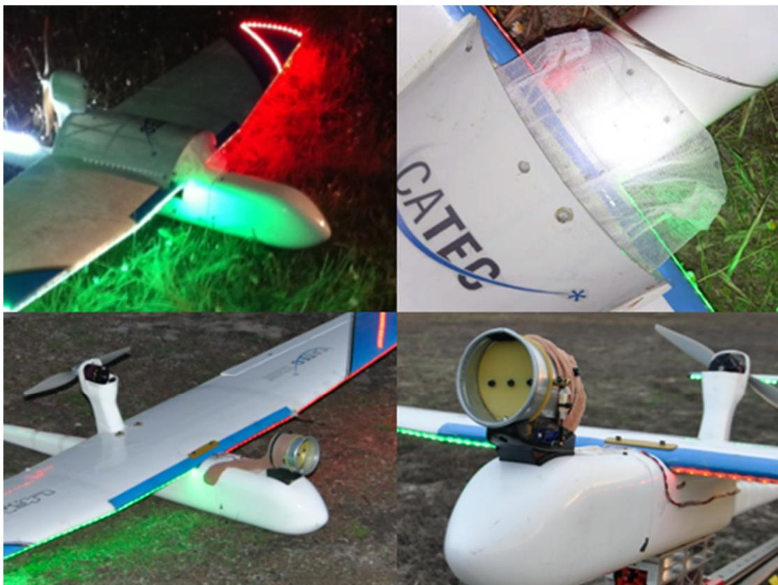
Figure 3. Insect traps details. Top: semiarch design; bottom: cylinder design.
