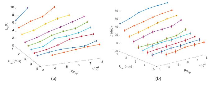
**Figure 6.** (a) Disturbance distance,  $L_b$  / R; and (b) jet angle,  $\beta$  for varying freestream speeds,  $U_{\infty}$  and varying  $Re_{tip}$  values.
