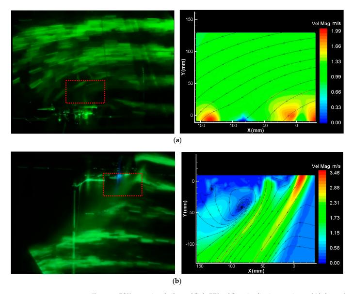
**Figure 11.** FOV comparison for forward flight PIV and flow visualization experiments (**a**) below and (**b**) above the multi-rotor UAV.
