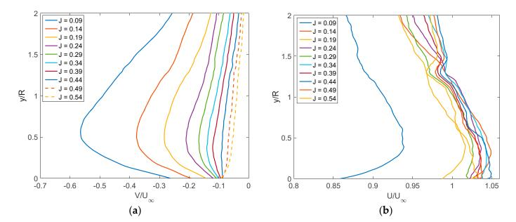
**Figure 15.** (a) Vertical velocity,  $V/U_{\infty}$ ; and (b) the horizontal velocity,  $U/U_{\infty}$  above the center of the multi-rotor UAV (x = 100 mm), with respect to y/R.
