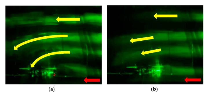
**Figure 9.** Flow visualization results above the multi-rotor UAV in forward flight at  $Re_{tip} = 8 \times 10^4$  for freestream speeds of (a)  $U_{\infty} = 3$  m/s (J = 0.12) and (b)  $U_{\infty} = 5$  m/s (J = 0.20).
