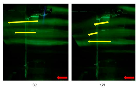
**Figure 4.** Flow visualization results from below the multi-rotor UAV in forward flight at  $U_{\infty} = 5$  m/s operating at (a)  $Re_{tip} = 3 \times 10^4$  (J = 0.54) and (b)  $Re_{tip} = 8 \times 10^4$  (J = 0.20).
