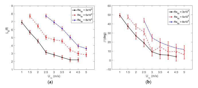
**Figure 5.** (a) Disturbance distance,  $L_b/R$ ; and (b) jet angle,  $\beta$  for select  $Re_{tip}$  as a function of  $U_{\infty}$ .
