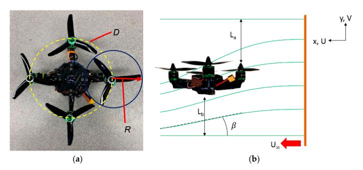
**Figure 2.** (a) The multi-rotor UAV used for all experiments including D, the diameter of the multi-rotor UAV and R, the radius of the propeller. (b) Multi-rotor UAV in simulated forward flight including the disturbance distance both below,  $L_b$  and above,  $L_a$  the multi-rotor UAV and the angle at which the flow is expelled from the front rotors,  $\beta$ .
