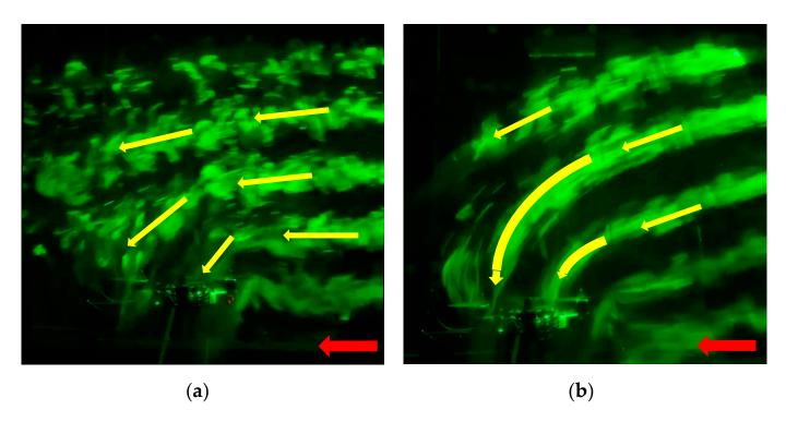
**Figure 8.** Flow visualization results above the multi-rotor UAV in forward flight at  $U_{\infty} = 1$  m/s and (a)  $Re_{tip} = 3 \times 10^4$  (J = 0.11) and (b)  $Re_{tip} = 8 \times 10^4$  (J = 0.04).
