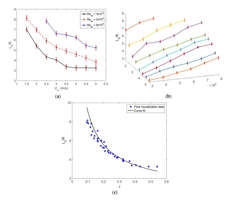
**Figure 10.** Disturbance distance,  $L_a/R$ , versus (a)  $U_{\infty}$ , (b)  $U_{\infty}$  and  $Re_{tip}$ , and (c) J from the flow visualization experiments.
