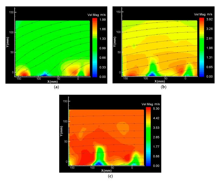
**Figure 14.** PIV results above the multi-rotor UAV in forward flight for (a) J = 0.09, (b) J = 0.24, and (c) J = 0.54.
