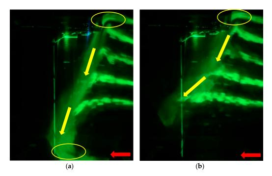
**Figure 3.** Flow visualization below the multi-rotor UAV in forward flight at  $U_{\infty} = 1$  m/s operating at (a)  $Re_{tip} = 8 \times 10^4$  (J = 0.04) and (b)  $Re_{tip} = 5 \times 10^4$  (J = 0.06).
