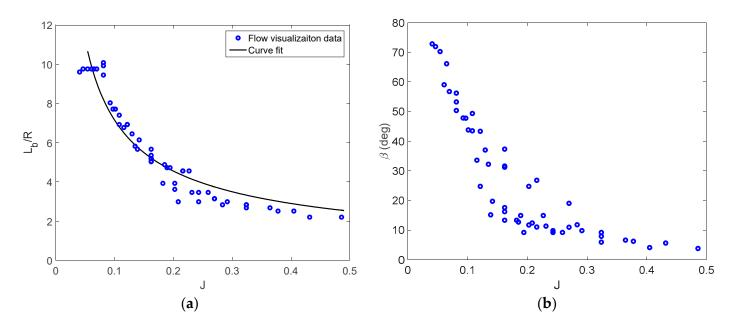
**Figure 7.** (a) Disturbance distance,  $L_b/R$ ; and (b) jet angle,  $\beta$  for varying advance ratios.
