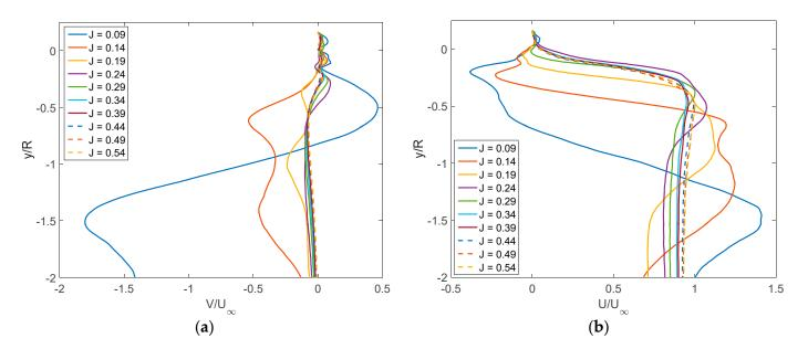
**Figure 13.** (a) Vertical velocity,  $V/U_{\infty}$ ; and (b) the horizontal velocity,  $U/U_{\infty}$  below the center of the multi-rotor UAV (x = 92 mm), with respect to y/R.
