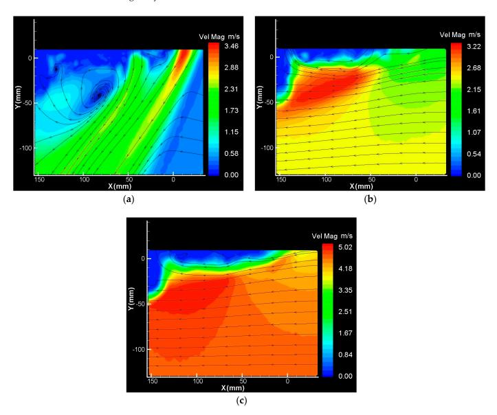
**Figure 12.** PIV results below the multi-rotor UAV in forward flight for (a) J = 0.09, (b) J = 0.24, and (c) J = 0.54.
