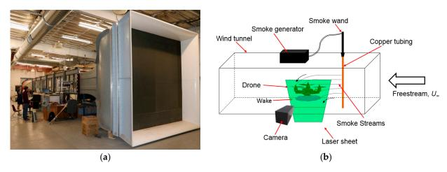
Figure 1. (a) NMSU wind tunnel and (b) schematic of flow visualization and PIV experimental setup.
