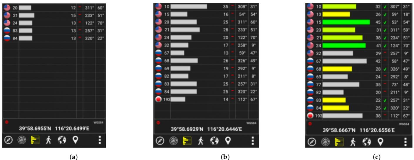
**Figure 5.** The status of visible satellites in three different environments. (a) Indoor. (b) Intermediate. (c) Outdoor.
