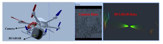
**Figure 9.** The simulation environment. The picture on the left is the UAV simulation platform equipped with virtual sensors, and the picture on the right is the virtual simulation scene.
