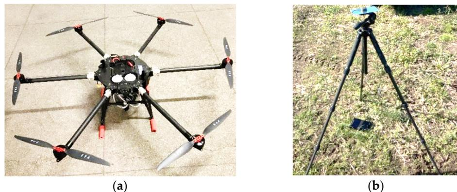
**Figure 2.** Equipment of the topographic surveying experiment. (a) UAV platform; (b) Base receiver of PPK-GNSS module.
