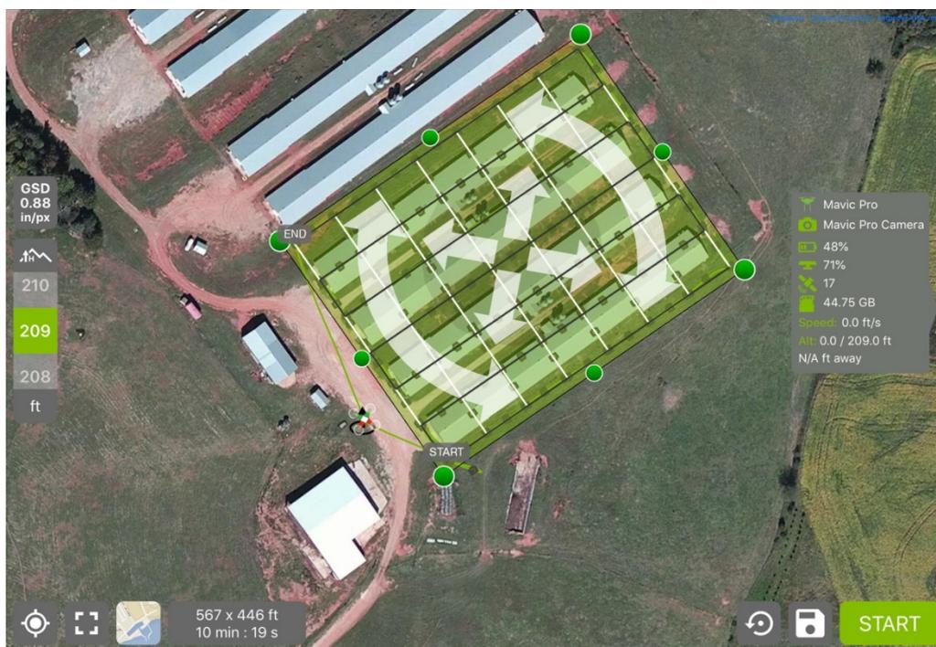
**Figure 1.** Sample image of the unmanned aerial vehicle (UAV) flight path in Pix4D Capture.
