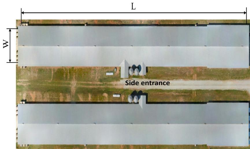
**Figure 2.** Poultry house viewed from above, illustrating length ( $L$ ) and width ( $W$ ) estimations observed from UAV images.
