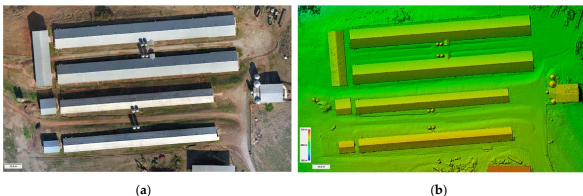
**Figure 6.** (a) Orthomosaic image ( $14,335 \times 11,647$ , 1.93 cm/px) and (b) digital surface model (DSM) ( $9548 \times 7884$ , 3.86 cm/px) built from dense point cloud (DPC).
