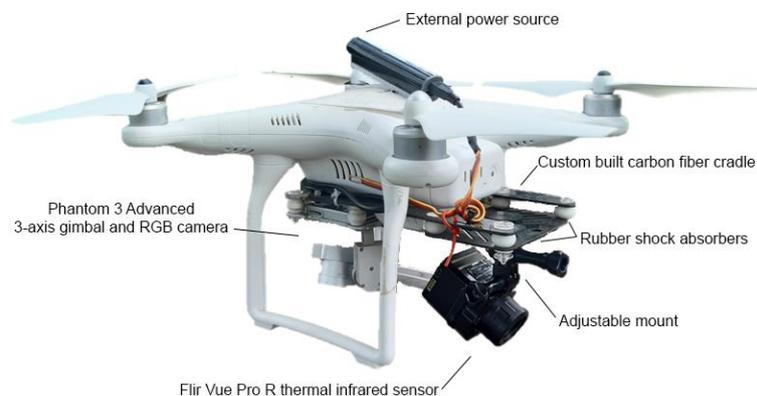
**Figure 1.** DJI Phantom 3 Advanced drone carrying a true-colour (RGB) camera and a Flir Vue Pro R (FVP) thermal infrared sensor fitted on custom cradle.
