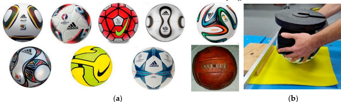
**Figure 1.** (a) The seven FIFA official match balls and two generic balls used for this study from right to left and up to down: Jabulani; Fracas; Ordem 3; Teamgeist; Brazuca; Kopanya; React; Finale 15; Vintage T-panel leather ball; (b) test set up with 10 kg mass on the ball, placed on a leather sheet on top of a force plate.
