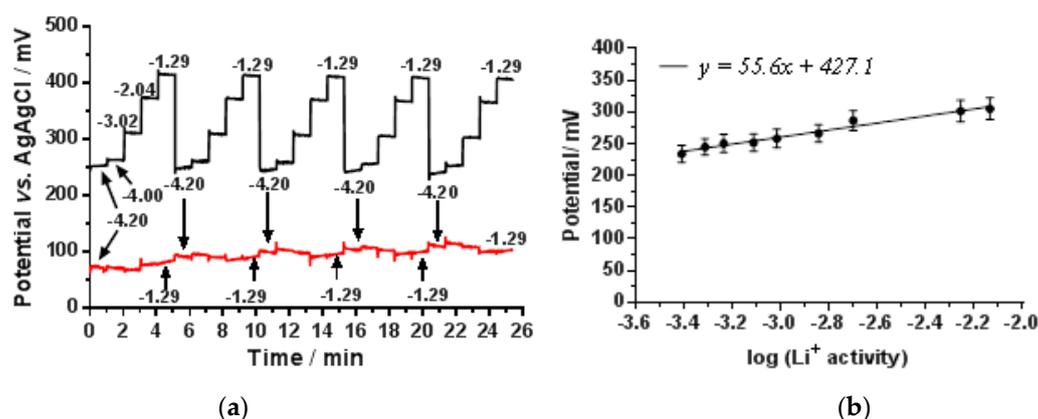
**Figure 3.** (a) The potentiometric response vs. time of the Li<sup>+</sup> sensor (black) and the fiber reference electrode (red) vs. Ag/AgCl double junction reference electrode with varying concentrations of LiCl solutions. The values on the plots are log (Li<sup>+</sup> activity); (b) the average potentiometric response of Li<sup>+</sup> sensor vs. the fiber reference electrode measured in LiCl solution (0.1–63.0 mM) in 0.1 ml spiked plasma (n = 5 devices).
