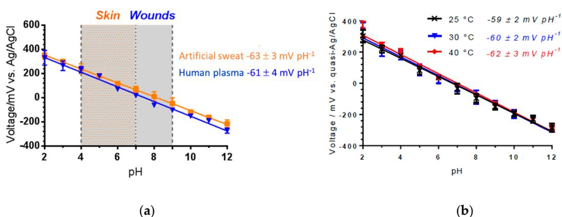
**Figure 2.** (a) Potentiometric response of Pani-PEDOT/MWCNT-cotton in pH adjusted artificial sweat and plasma.  $N = 3$ ; (b) potentiometric response of Pani-PEDOT-MWCNT-cotton in buffered solutions of varying pH levels between 25 and 40 °C,  $n = 3$ .
