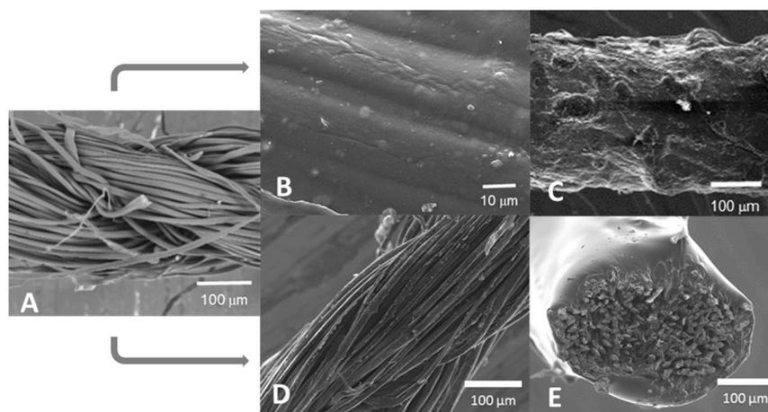
**Figure 1.** SEM images of cotton thread (A), PEDOT/MWCNT-cotton (B), Pani-coated PEDOT/MWCNT-cotton (C), SWCNT-cotton (D), cotton-based Li<sup>+</sup> sensor (E).
