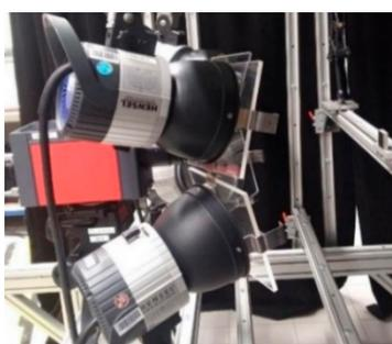
**Figure 1.** Setup for pulsed thermography with four flash lamps.
