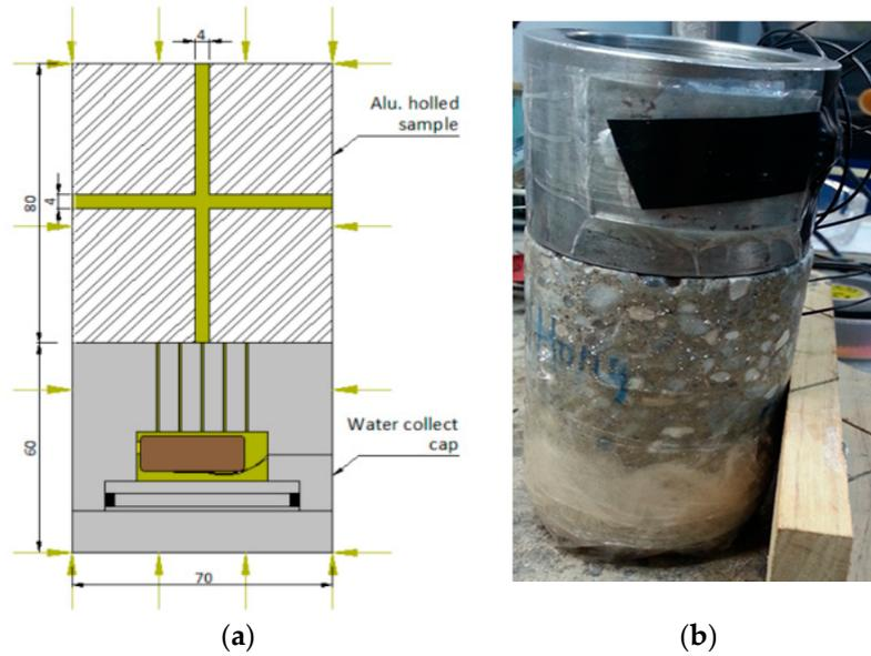
**Figure 3.** Experimental set up: (a) calibration test concept (b) pore pressure test preparation.
