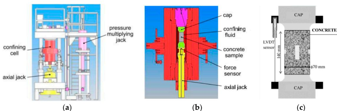
**Figure 1.** GIGA press (a) general view (b) section of the confining cell (c) sample instrumentation.
