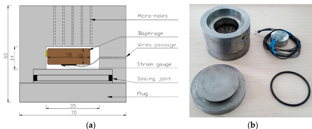
**Figure 2.** Water collecting cap with the sensor of hydrostatic type (a) design and (b) real concept.
