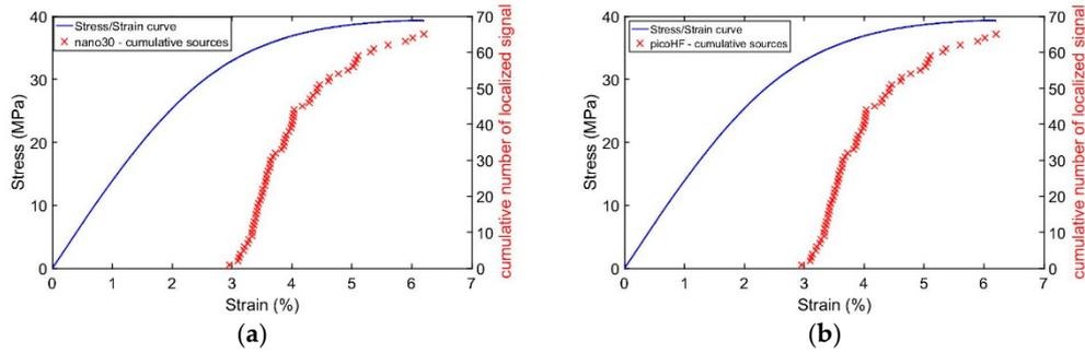
Figure 5. Cumulative localized signal during SFFT: (a) sources located by nano30; (b) by picoHF.
