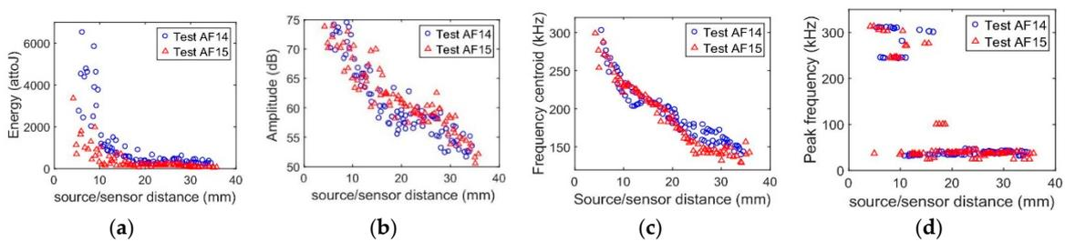
Figure 6. Temporal descriptors vs. source/sensor distance: (a) energy in attoJ, (b) amplitude in dB, (c) frequency centroid in kHz and (d) peak frequency in kHz.
