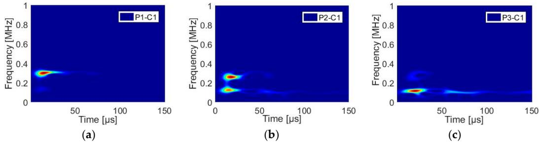
**Figure 8.** Time-frequency results calculated using smoothed pseudo Vigner-Ville distribution for 3 source positions for signals recorded on C1: (a) P1 position, (b) P2 position and (c) P3 position
