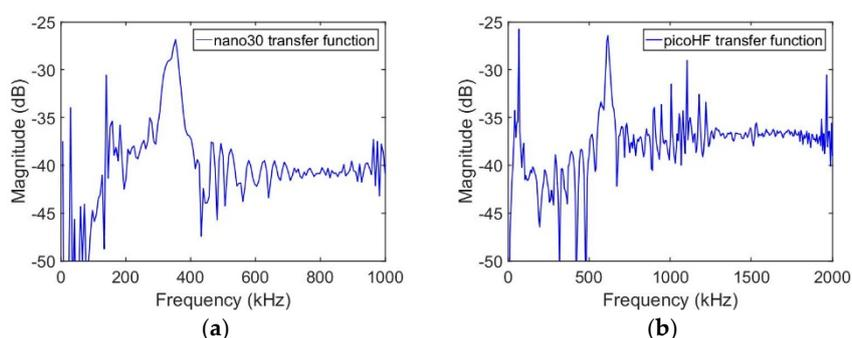
**Figure 3.** Transfer function of (a) nano30 and (b) picoHF, determined by reciprocity method.
