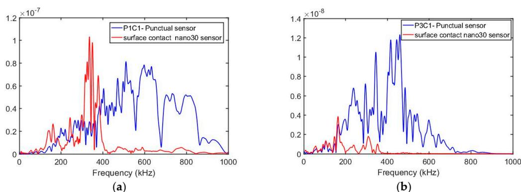
**Figure 10.** Comparison between simulated punctual sensors, surface contact sensors. (a) Signals of simulated fiber break at P1 position at C1 sensor; (b) at P3 position at C1 sensor.
