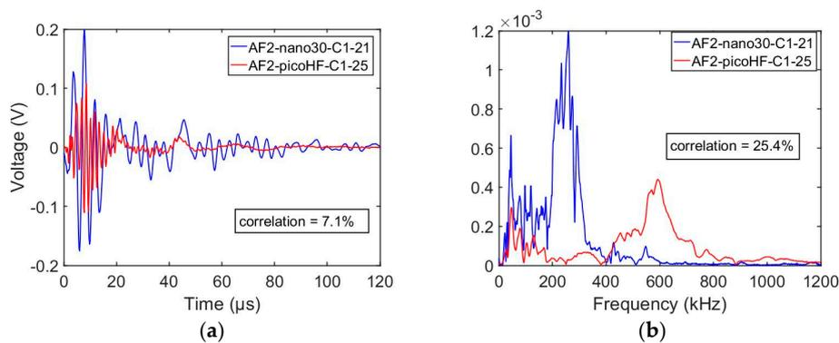
**Figure 9.** Temporal signals (a) and frequency spectra (b) for two types of sensors.
