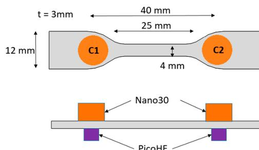
Figure 1. Dimension of specimen and sensors placement.
