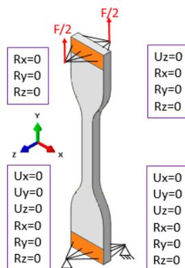
Figure 2. Scheme of the numerical specimen with the boundary conditions.
