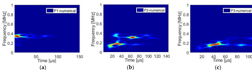
**Figure 11.** Numerical results: time frequency calculated with smoothed pseudo Vigner-Ville distribution for three source positions: (a) P1 position, (b) P2 position and (c) P3 position
