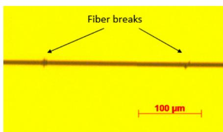
**Figure 4.** Fiber breaks as observed by optical microscopy.
