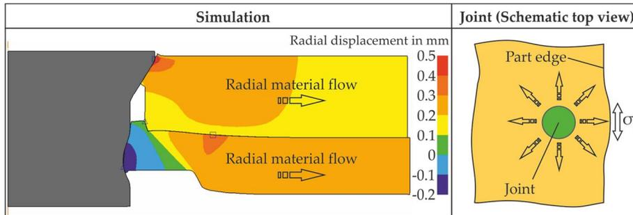
**Figure 4.** Formation of tangential tensile stresses at the part edge through SPR-S.
