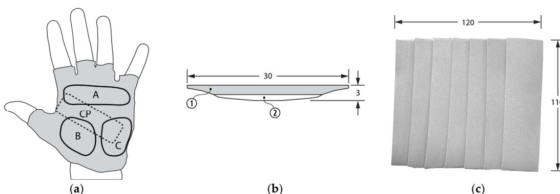
**Figure 2.** (a) Palm side of tested gloves model with identification of padded areas (A, B, C) and of the contact patch between the glove and the instrumented brake hoods (CP); (b) Bar tape cross-section. 1-ethylene-vinyl acetate (EVA) foam; 2-elastomer gel layer; (c) Handlebar tape strips arrangement. Note: All dimensions are in mm.
