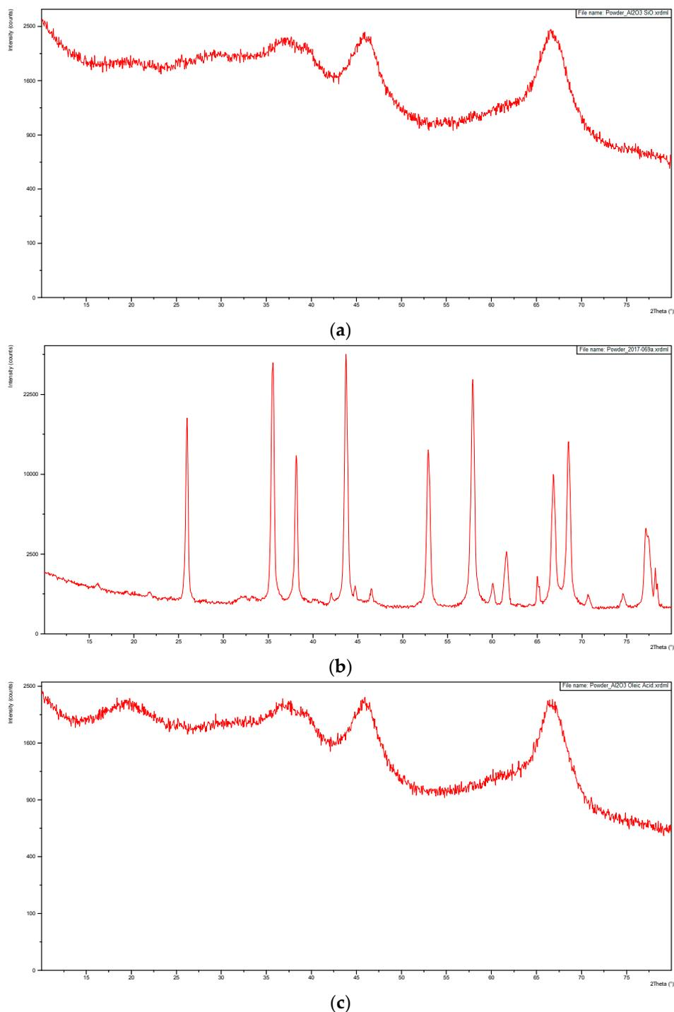
**Figure 4.** XRD patterns for Al<sub>2</sub>O<sub>3</sub> NPs (a) bare (b) coated with OA (c) coated with SiO<sub>2</sub>.
