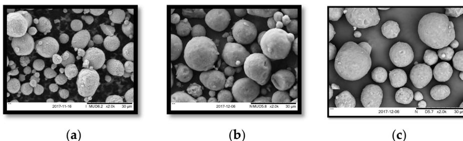
**Figure 2.** SEM images of  $\text{Al}_2\text{O}_3$  NPs (a) before coating (b) after coating (OA) (c) after coating ( $\text{SiO}_2$ ) at 2000 $\times$  magnification.
