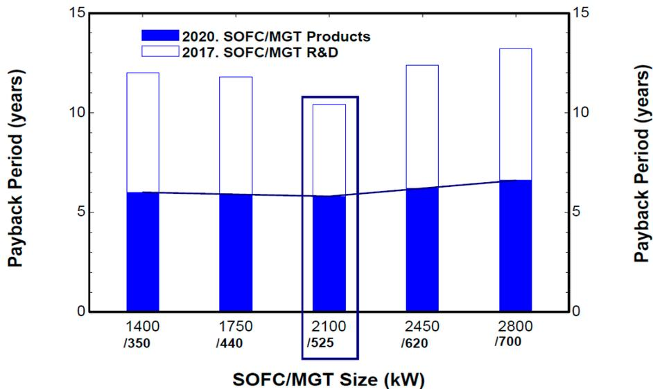
Figure 3. Payback period of the optimal SOFC/MGT system.
