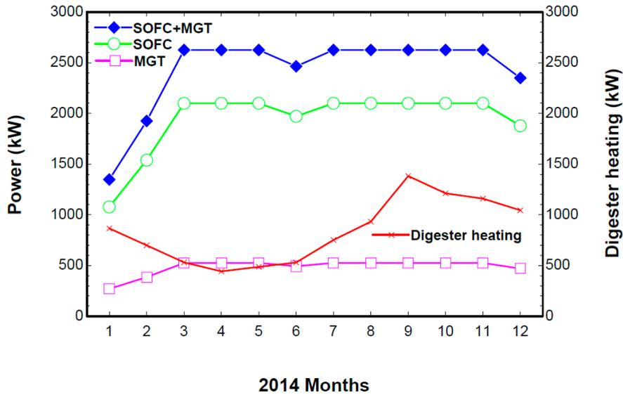
Figure 2. Operating characteristics of SOFC/MGT in 2014.
