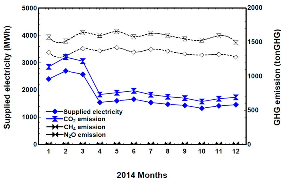
Figure 4. Electricity consumption and Greenhouse gas of SOFC/MGT in 2014.
