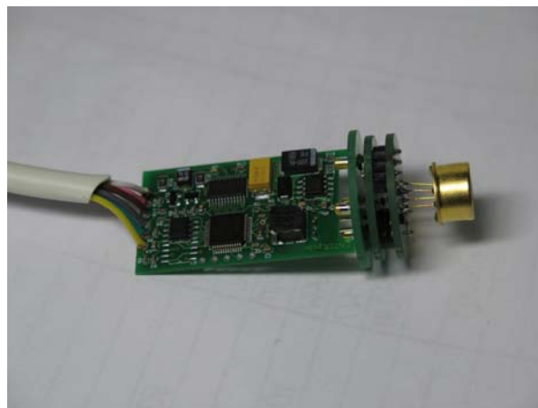
Figure 6. Smart sensor unit with gas sensor in TO-8 packaging. The round board is a smart unit with UART interface enabling temperature control of the sensor and providing all information about concentration of gas, type of sensor, enabling compensation of ambient humidity, etc. Diameter of this board is of 25 mm.
