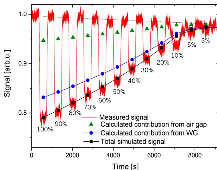
**Figure 2.** Measured signal at the detector (red solid line) for the gas concentrations indicated in the plot. Triangles and circles are the change in transmittance (calculated according to the Beer-Lambert law) due to absorption in the air gap and of the waveguide evanescent field, respectively. Square symbols show the calculated total signal accounting for both effects
