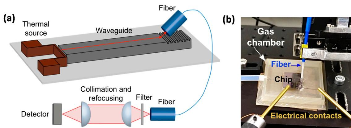
**Figure 1.** (a) Schematic view of the measured structure and of the measurement setup; (b) Experimental realization of the gas cell, with access for the electrical contacts and the fiber.
