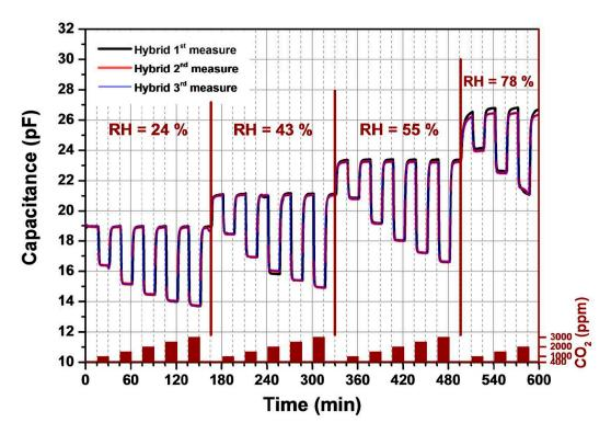
**Figure 2.** Capacitance response versus time of amine functionalized silica nanoparticles based CO<sub>2</sub> sensor. Capacitance change recorded under different CO<sub>2</sub> concentrations and relative humidity levels.
