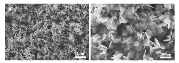
**Figure 1.** FE-SEM images of the as-synthesized rGO@ZnO<sub>1-x</sub> composites with low (**a**) and high (**b**) magnifications.
