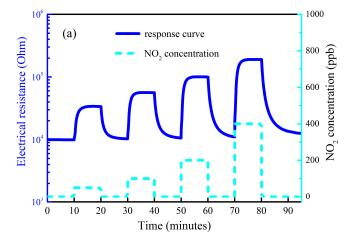
**Figure 4.** The electrical resistance of the rGO@ZnO<sub>1-x</sub> nanocomposites versus NO<sub>2</sub> gas in 50, 100, 200 and 400 ppb illuminated by white light at room temperature.
