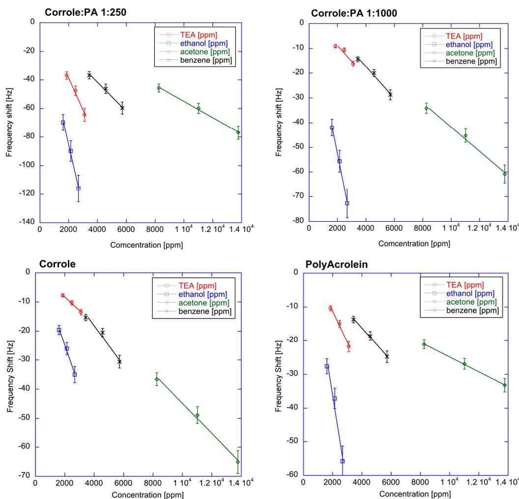
**Figure 3.** Response curve of four QMBs coated with corrole functionalized polyacrolein at two different acrolein:corrole ratios (1:250 and 1:1000), and two sensors coated with either corrole or polyacrolein.
