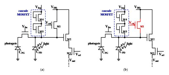
**Figure 1.** Schematic diagrams; (**a**) conventional linear-logarithmic pixel and (**b**) proposed linear-logarithmic pixel.
