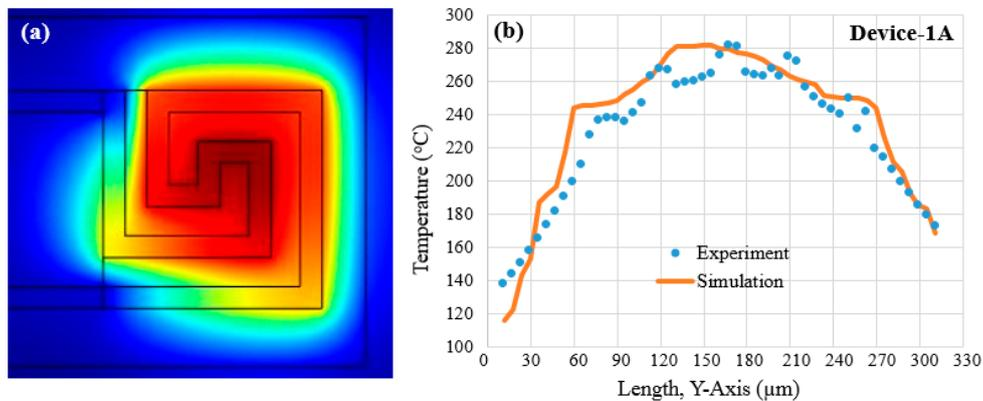
**Figure 3.** (a) Representative simulation of double meander micro-hotplate (device 1A),  $281^\circ\text{C}$  at 28 mW; (b) Temperature distribution along  $y$ -axis for simulated and experimental values of micro-hotplate "1A" at  $281^\circ\text{C}$ .
