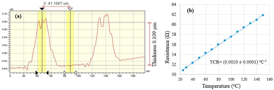
**Figure 2.** (a) Optical profilometry of the printed Au printed patterns; (b) Resistance as a function of temperature (TCR) for Au micro-hotplates on PI, ( $\text{TCR} = 0.0020 \pm 0.0001/^\circ\text{C}$ ).
