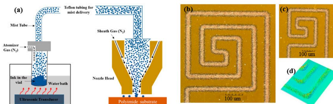
**Figure 1.** (a) Schematic of Ultrasonic Atomizer jet printing system; (b) Double meander micro-hotplate  $500 \times 500 \mu\text{m}^2$ ; (c)  $300 \times 300 \mu\text{m}^2$ ; (d) Optical graph of surface profile.
