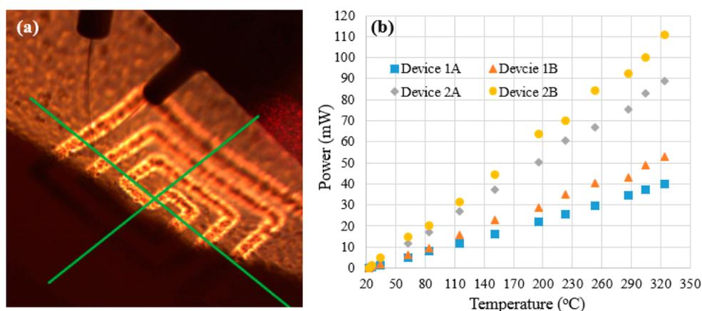
**Figure 4.** (a) Thermal scanning for temperature measurement, (b) Power consumption against temperature.
