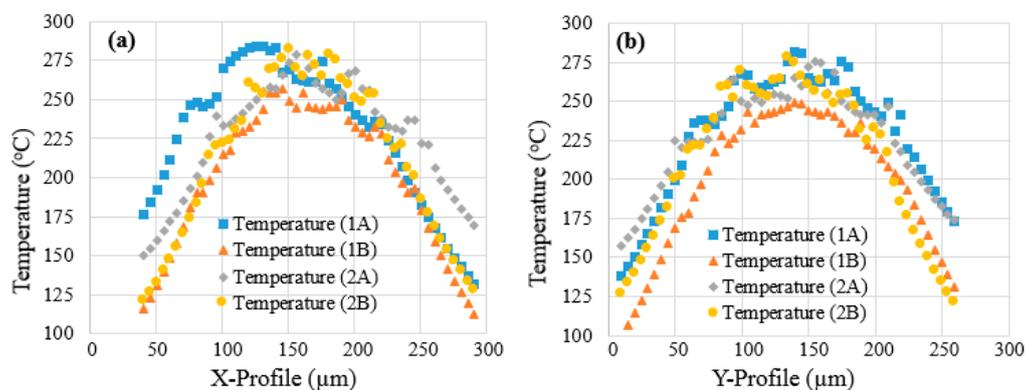
**Figure 5.** Experimental values of temperature distribution at 270 °C on (a) *x*-axis (b) *y*-axis of micro-hotplates.
