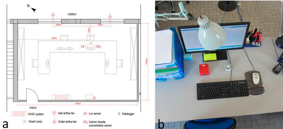
**Figure 2.** Installation in working conditions: (a) plan of the office; (b) workstation with smart lamp and sensors.
