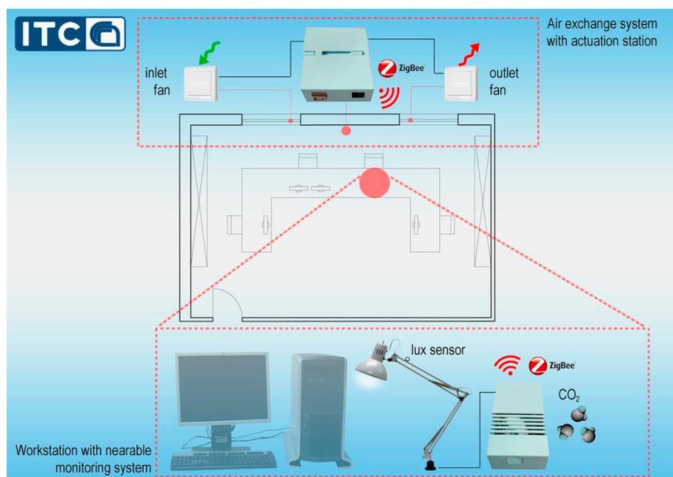
**Figure 1.** Hardware layout in a real case study.
