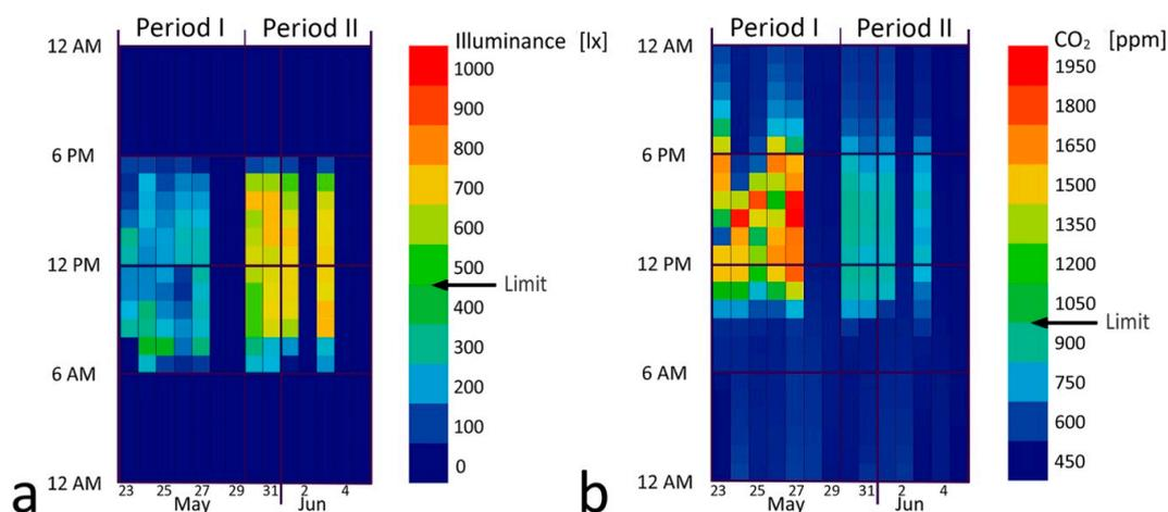
**Figure 3.** Hourly average data for manual control (period I, 23–29 May) and automatic control (period II, 30 May–5 June): (a) illuminance level; (b) CO<sub>2</sub> concentration.
