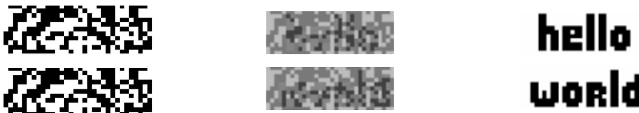
**Figure 11.** Multiple trigger images for a “hello world” example. A sequence generated by rule set  $f_6$ . Left: the middle section of the bias image (shown twice). Middle: the corresponding sections of the first and second trigger images. Right: the target afterimage patterns ( $a_1$ ,  $a_2$  as before). This sequence also demonstrates the effects of scrambling when using finer target shapes.
