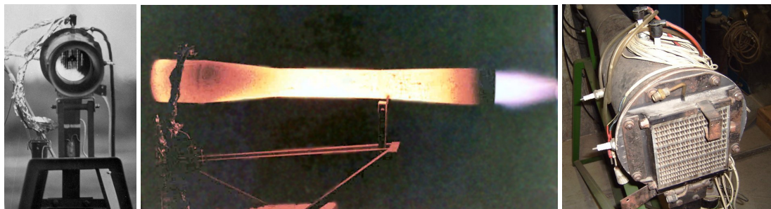
Figure 1. Pulse combustion application: the Schmidt-Argus pulse jet engine in action. Thrust tests led at Thalerhof airport by Zhuber and Pirker in the 1960s (archives TU Graz/TTM) with detail of the Reed air valve and ignition sparklers.
