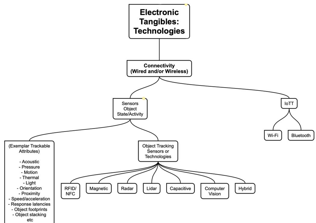
**Figure 7.** Object tracking technologies.
