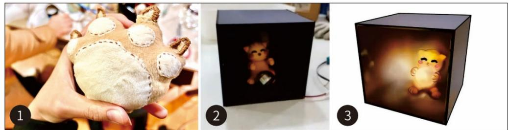
**Figure 2.** *Personal Interaction Devices in Car* technical prototype ((1) Triggering haptic feedback of the toy by pat and press; (2) the general status of the display device; (3) the indication state of the display device with visual feedback and auditory feedback).
