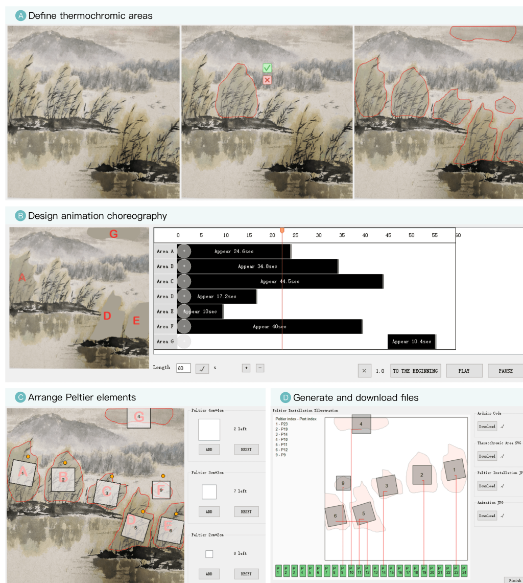
Figure 4. The step-by-step user interfaces and workflow of the design tool: ((A), top) users easily design areas that need to have a thermochromic effect; ((B), middle) users design and preview the choreographing animation; ((C), bottom left) users can try different layout designs of three types of Peltier elements; ((D), bottom right) users download three files to facilitate the creation process: an SVG line-drawing file to process the thermally conductive layer, a piece of Arduino code to control heating/cooling, and a Peltier installation guidance.
