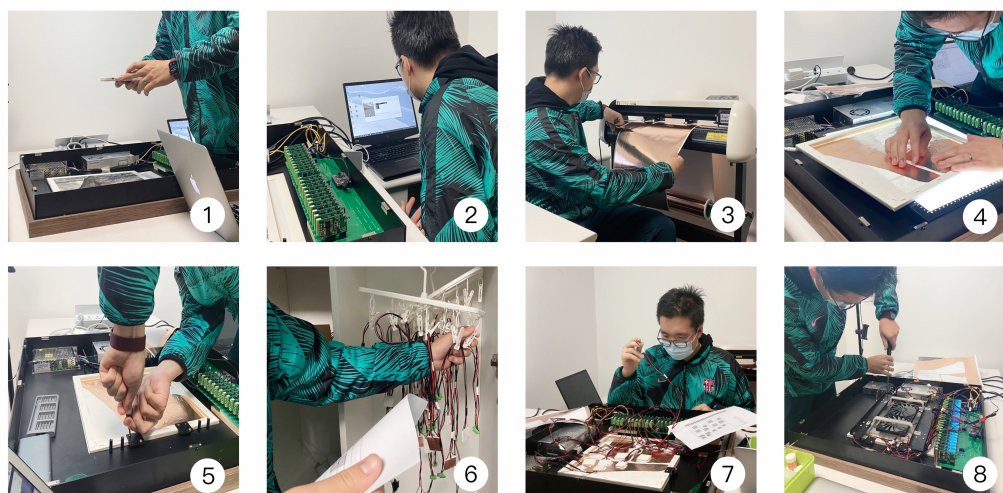
Figure 10. The use process of the toolkit: steps 1–2, design tool operation; steps 3–4, make the thermally conductive layer; steps 5–8, assemble the hardware components, including (5) the inner wooden picture frame, (6–7) the Peltier elements, and (8) the heat dissipation device.
