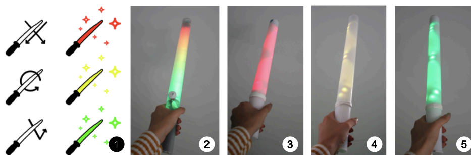
Figure 6. Glowing Wand technical prototype (1. different hand gesture designs; 2. switch for a rainbow feedback; 3. negative tick gesture to red light; 4. circle gesture to yellow light; 5. tick gesture to green light).
