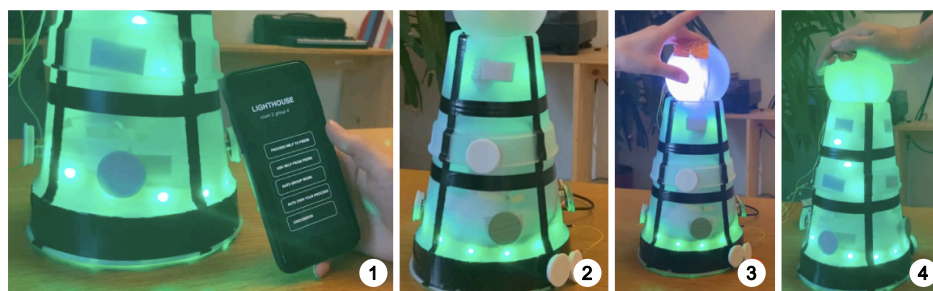
Figure 5. Tower technical prototype (1. use app to communicate with other groups; 2. place magnets on the Tower to choose an answer, green means I am confident , white means I am not sure ; 3. rotate top bulb to seek help; 4. touch top bulb to finish the activity).
