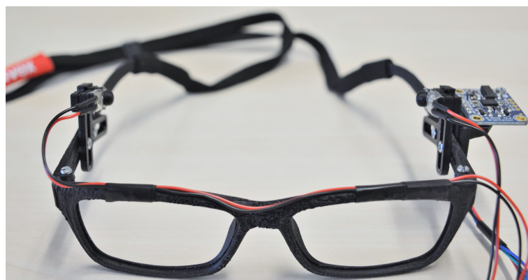
Figure 3. Image of the mouse alternative. The inertial measurement unit that tracks head motions for mouse cursor control is shown on the right. Force-sensing resistors are mounted onto each temple and can be adjusted in position to ensure good contact with the Temporalis muscle for mouse click activation. The spectacle strap is used to avoid involuntary movement of the spectacles caused by head motions or the activation of the Temporalis muscle.
