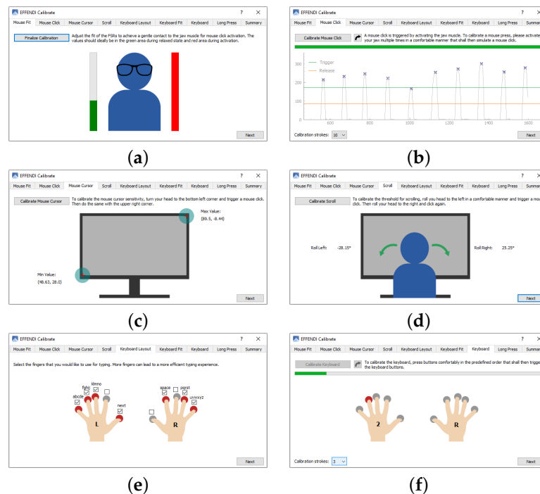
Figure 8. User interface during the guided calibration process. (a) Calibration of the force between the sensor and the Temporalis muscle. (b) Calibration of the threshold to activate a mouse click. (c) Calibration of the cursor sensitivity based on screen size. (d) Calibration of thresholds for scrolling. (e) Calibration of the keyboard layout based on usable fingers. (f) Calibration of the duration from a long button press.
