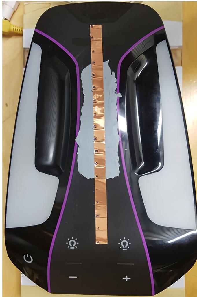
**Figure 7.** The control panel top view. The central slider is filled in with Blu Tack for Measurements to be completed using the MicroSense sensor.
