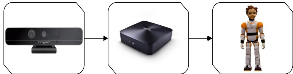
**Figure 1.** Experimental setup. Starting from the left: Intel® RealSense™ (model F200), computer and ZECA robot.
