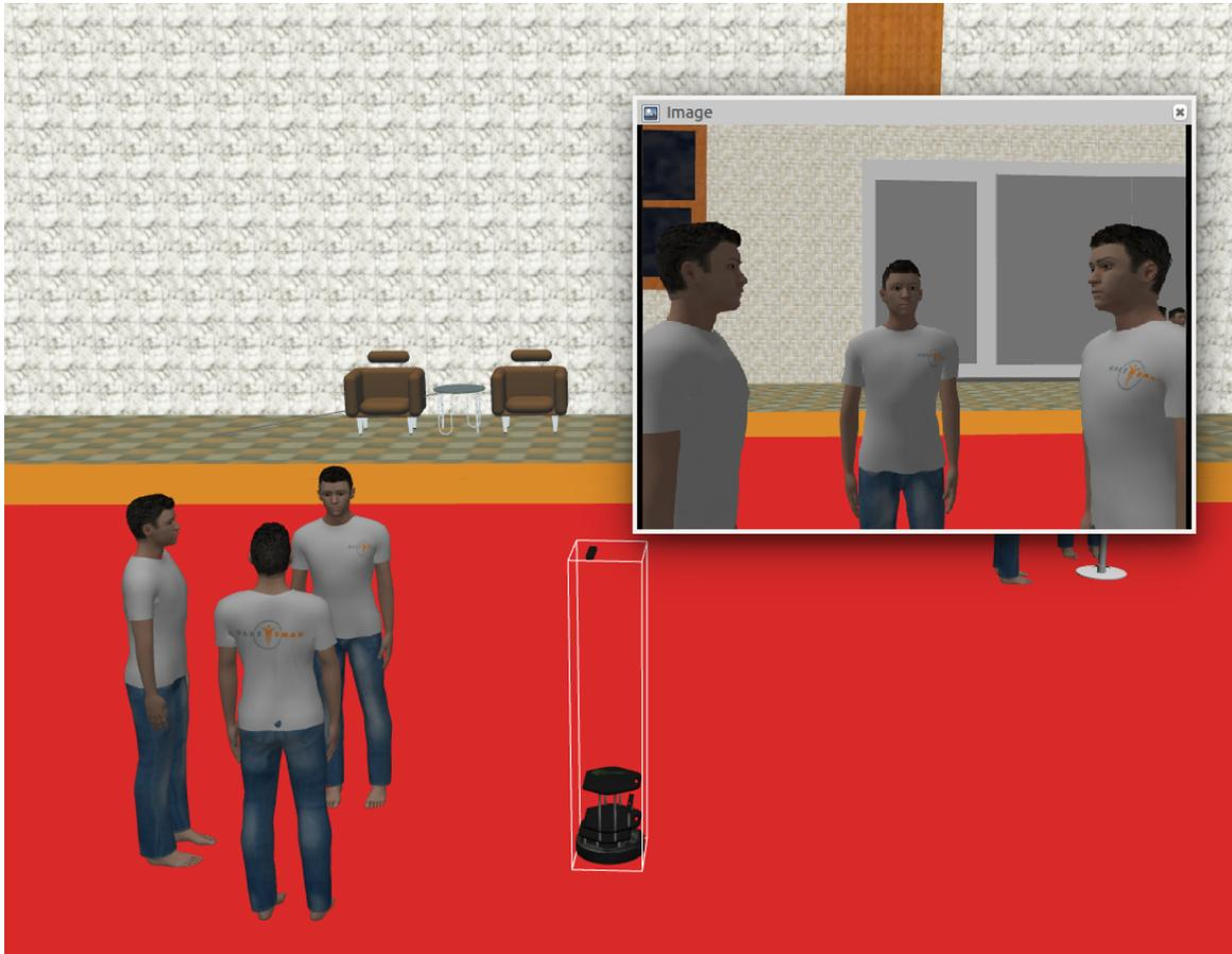
**Figure 6.** Image showing VAs interacting with each other and a modified TurtleBot observing. The inside image shows the view from the robot's sensory system. This is the egocentric view seen by the subject while teleoperating a robot.
