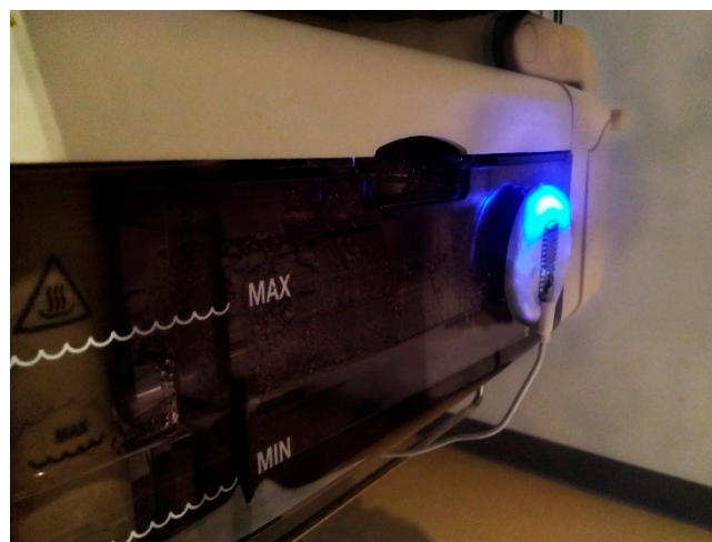
Figure 1. CheckMate attached to one of the medical devices; the water container of an incubator.
