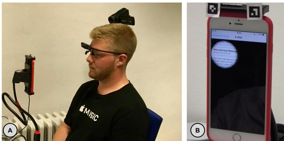
**Figure 2.** The figure shows the usability study's setup. The iPhone was mounted on a holder such that it was 30 cm away from the user's eyes (A). From the user's perspective, they could see the phone with the spot moving according to the user's gaze (B).
