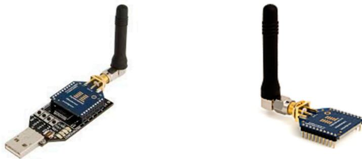
Figure 4. XBee RF Module and USB PC Gateway.
