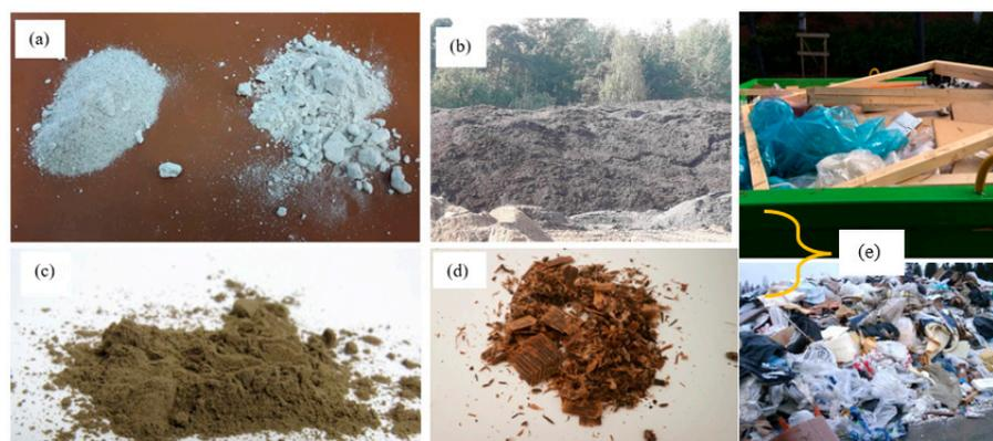
**Figure 1.** Industrial waste side streams used in this study: (a) fine and coarse fraction of flotation sand; (b) green liquor sludge; (c) paper mill power plant ash; (d) fiber waste; (e) mixed composition of materials in CDW.
