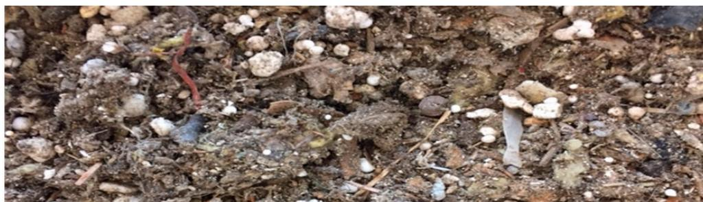
**Figure 4.** Screen reject from mixed CDW.
