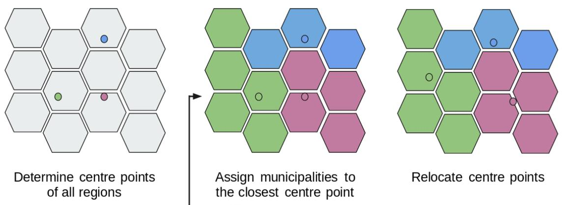
**Figure 1.** Visual representation of the steps taken to assign municipalities to spatially clustered regions using the k-means algorithm. This algorithm can be applied to generate different numbers of regions. This number of regions is controlled by the variable  $k$ . To be able to compare the generated regions with a certain set of identity regions, this  $k$  is set equal to the number of regions present in this set of identity regions.
