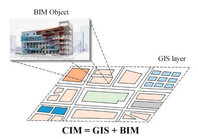
Figure 4. CIM integration of BIM and GIS [36].
